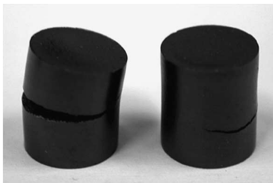
Fig. 3. UO 2 pellets sintered at high heating rates of 20 K/min (left) and 30 K/min (right).
